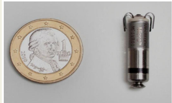
Figure 2 The Medtronic Micra™ Transcatheter Pacing System (reproduced with permission from Medtronic Inc.).
